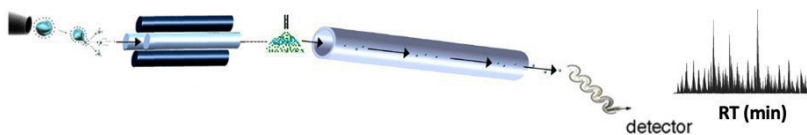
Figure 6.2 Sample preparation and LC are similar with targeted and untargeted approaches, the primary distinguishing feature is the instrument used. For targeted, typically triple quadrupoles are used and for untargeted, either QTOFs or orbitraps.
