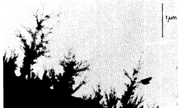
Fig. 3. Electron micrograph of a 3 \mu\text{m} platinum wire activated with acetone at a pressure of 3 \times 10^{-3} torr and an anode-cathode voltage of 10 kV.
