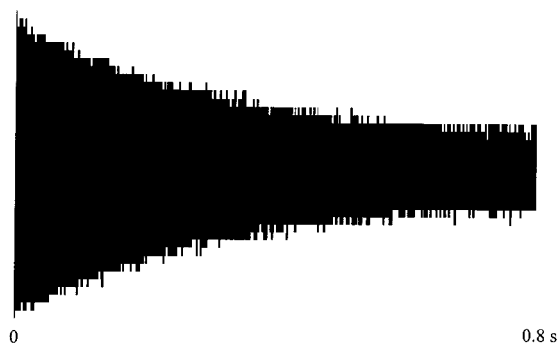
Figure 6. Typical transient for ^{56}\text{Fe}^+ . Hundreds of thousands of oscillations merge into the black envelope.
